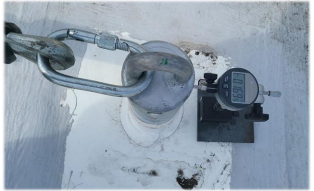
Measuring Anchorage Movement During Testing
