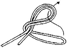
Step 3. After going over the top, come around the bottom of the rope with the loop and then from over the top insert the end of the loop into the first loop. This will look like a figure 8. Pull this tight. It is recommended to insert a "thimble" into this loop for ease of using locking D rings and for protection of the rope.
