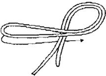
Step 2. Take the middle of that loop and make another loop in the rope that is at least 18" in length. Now you have a doubled loop in the end of the rope. Take the end of the loop and go over the top of the doubled rope.
