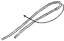
Step 1. Take the end of the rope and make a single loop at least 24" (2') in length.
